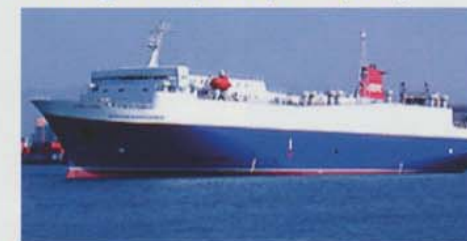
● RORO ship: 7,389 tons gross ● Speed: 20 knots ● Carrying capacity: 240TEU
